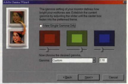
Adobe gamma menu installed with Adobe Photoshop 6.0. Menu loads in monitor profile, set contrast, gamma, phosphors and white point.
