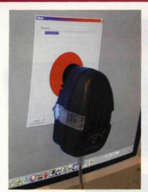
The X-rite Monitor Optimizer with software program is used to create monitor profiles.
