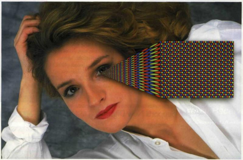
Corel stock photo image with small section of computer screen enlarged. Full red, green and blue make up white on the computer monitor.
